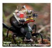
Scientists have developed a tiny camera that can be put on the back of a beetle. The camera can record where the bug goes. This will give the scientists a bug's-eye view of the world. The researchers want to use the camera to
